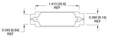
For back shell assembly applications: ONLY use the mounting screws when mounting slide lock bar DO NOT use the flat washers, lock washers, and #4-40 nuts
